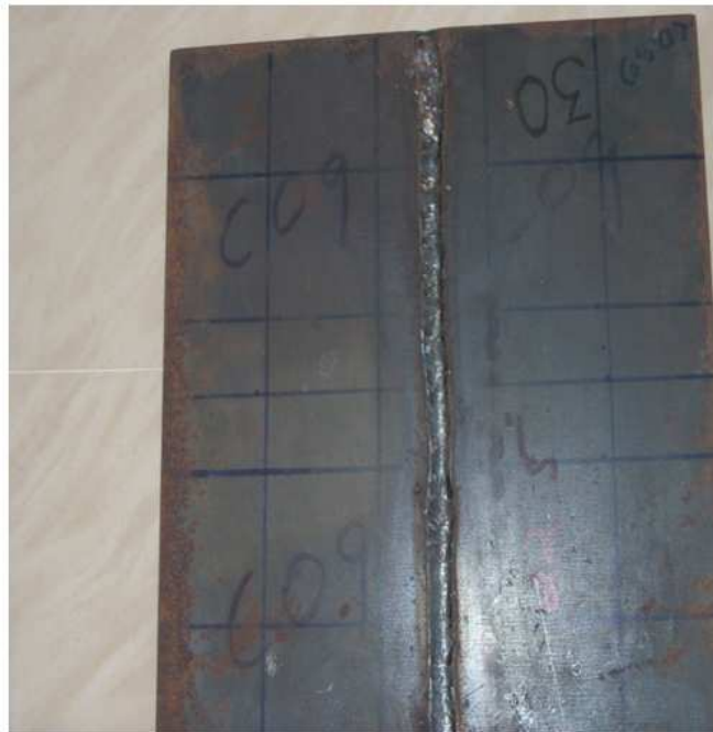
Figure 1.5: Specimen Welded Using CO 2 Arc Welding
